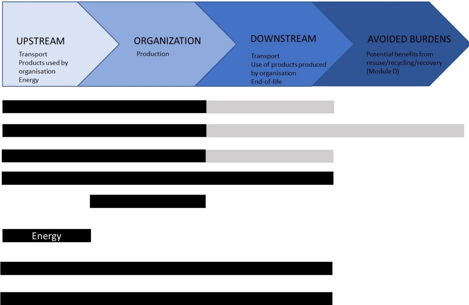
Figure 2 Illustration of how the different standards and frameworks relates to the *system boundaries* (life cycle phases). Solid black symbolizes mandatory life cycle phases, while grey illustrates optional life cycle phases.
