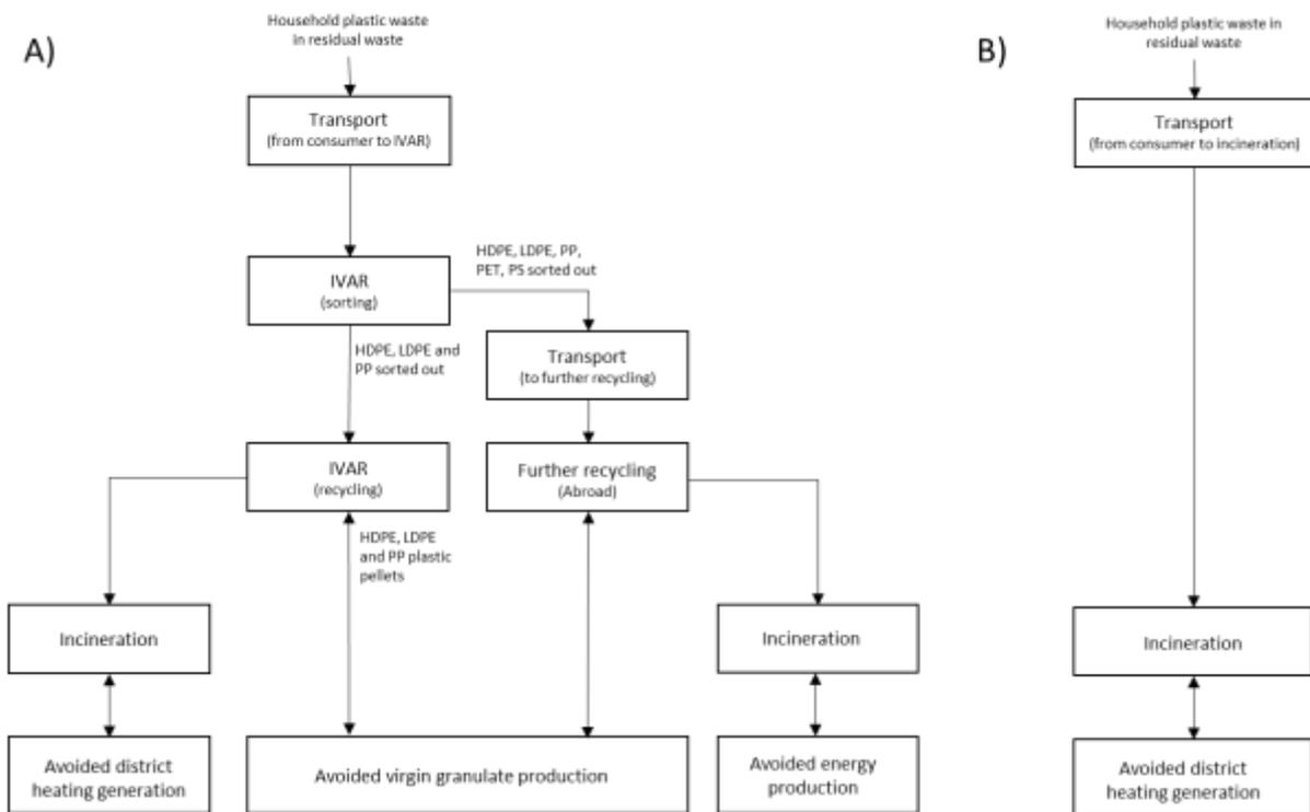
**Figure 3.** Simplified flowchart for a) household plastic waste sorted and recycled at IVAR and b) household plastic in residual waste going to incineration instead of sorting and recycling at IVAR.
