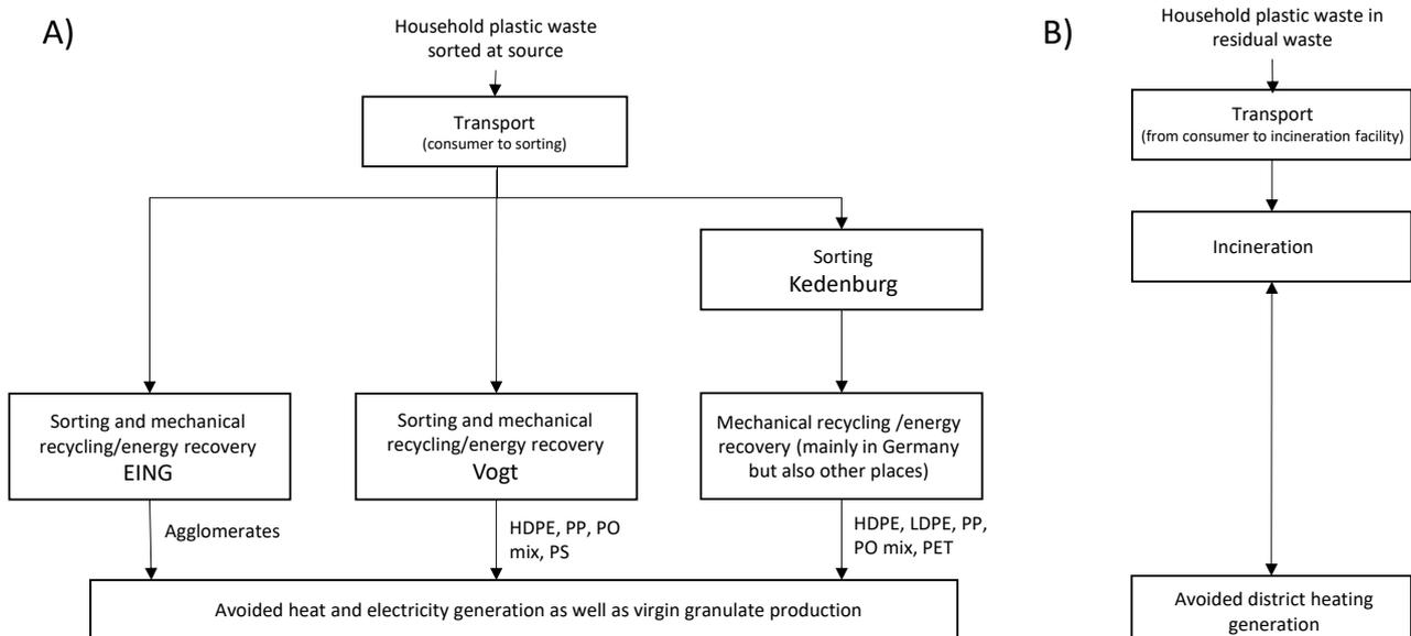
**Figure 1.** Simplified flowchart for the two compared systems A) household plastic waste sorted at source and B) household plastic waste in residual waste sent to incineration with energy recovery
