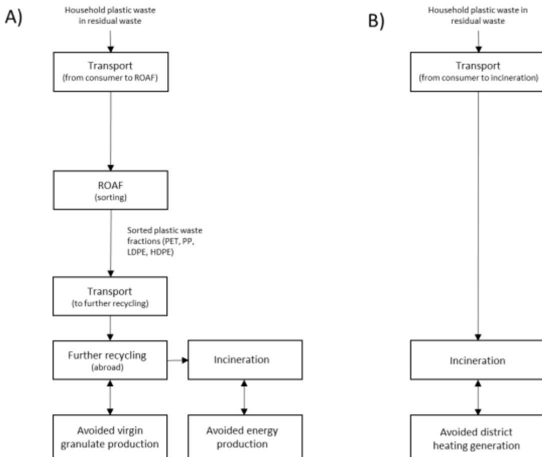
**Figure 2.** Simplified flowchart for the compared systems a) household plastic waste sorted at ROAF and further recycling abroad and b) household plastic waste going to incineration together with the residual waste instead of sorting at ROAF.
